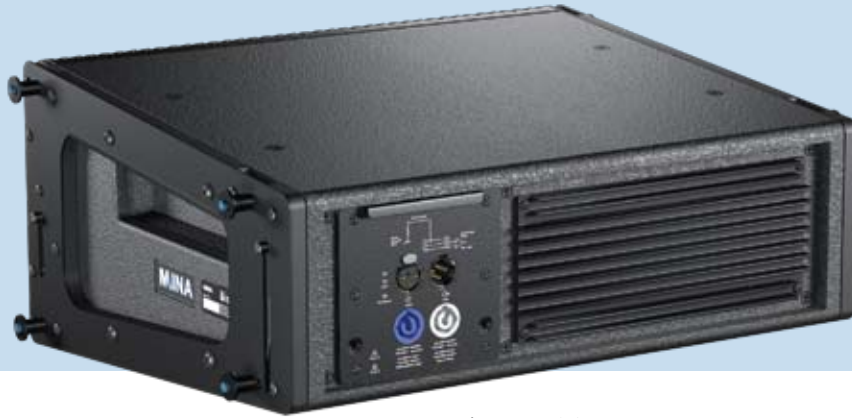
MINA's powerful three-channel Class-D amplifier
